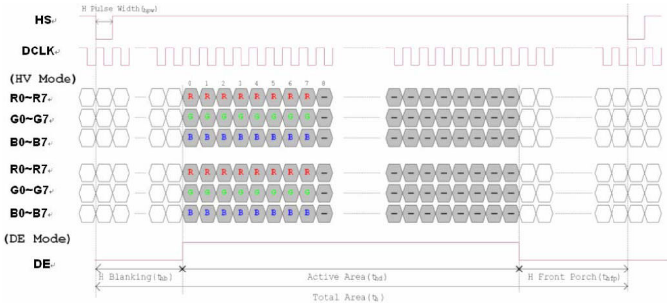
Figure 3.1 Horizontal input timing diagram
